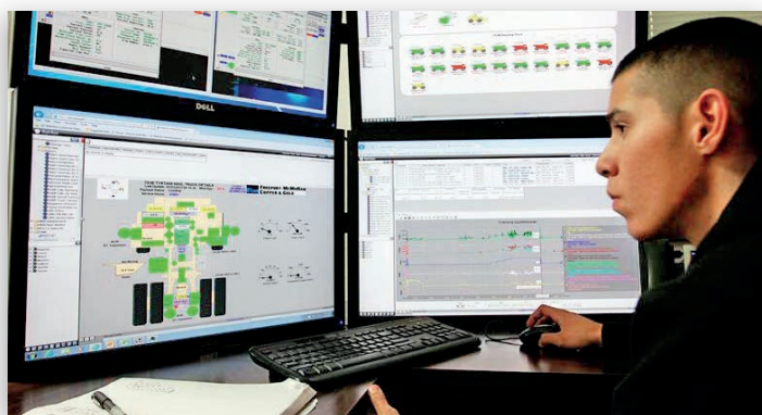
Tyrone mine diagnostic mechanic, Royce Parra, conducts real-time performance monitoring of heavy mining equipment using Remote Access Monitoring Process (RAMP) technology. Implementation of RAMP has resulted in improved fleet reliability through detection and prevention of premature equipment failure, as well as the promotion of operating behaviors that safely increase the efficiency of material movement.
